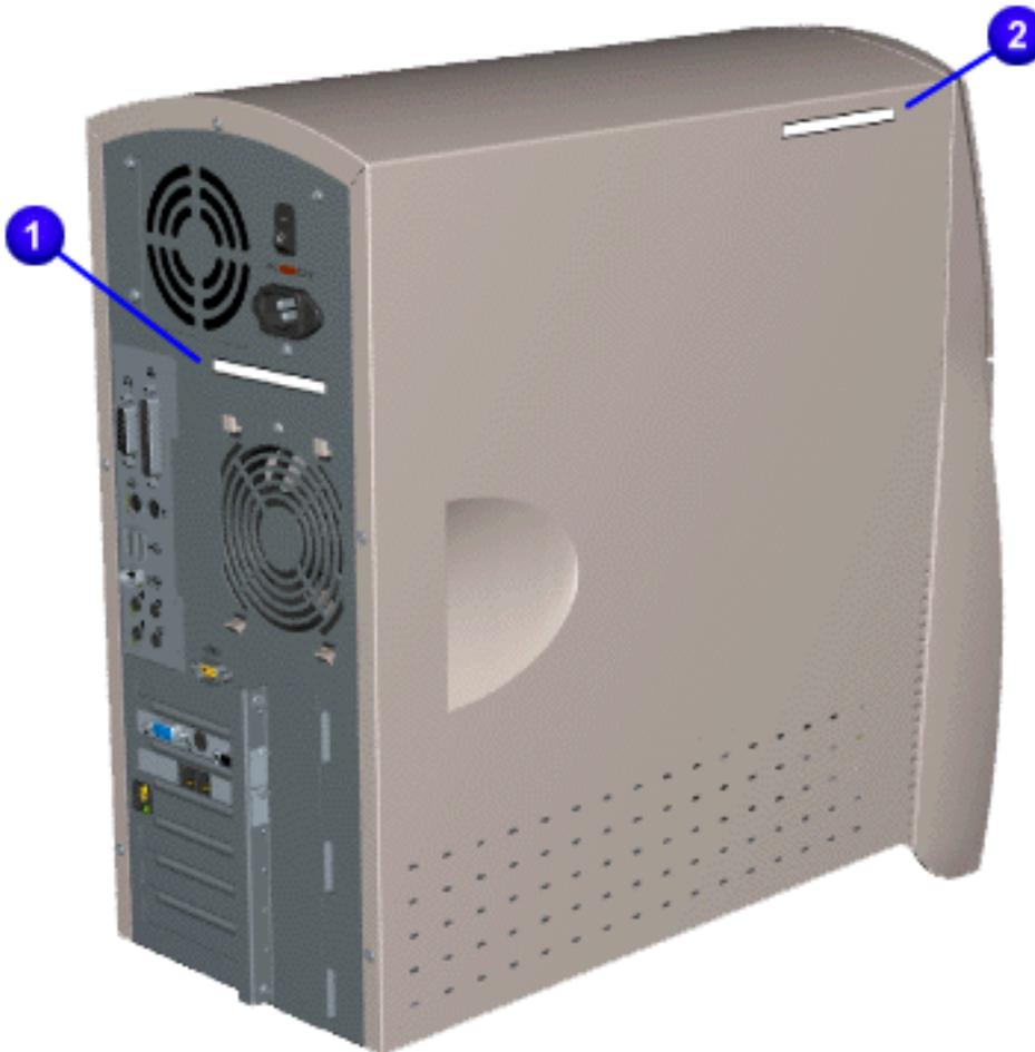
The computer serial number should be provided to Compaq whenever requesting information or ordering spare parts. The serial number is located on the rear **1** and left **2** side of the computer.
