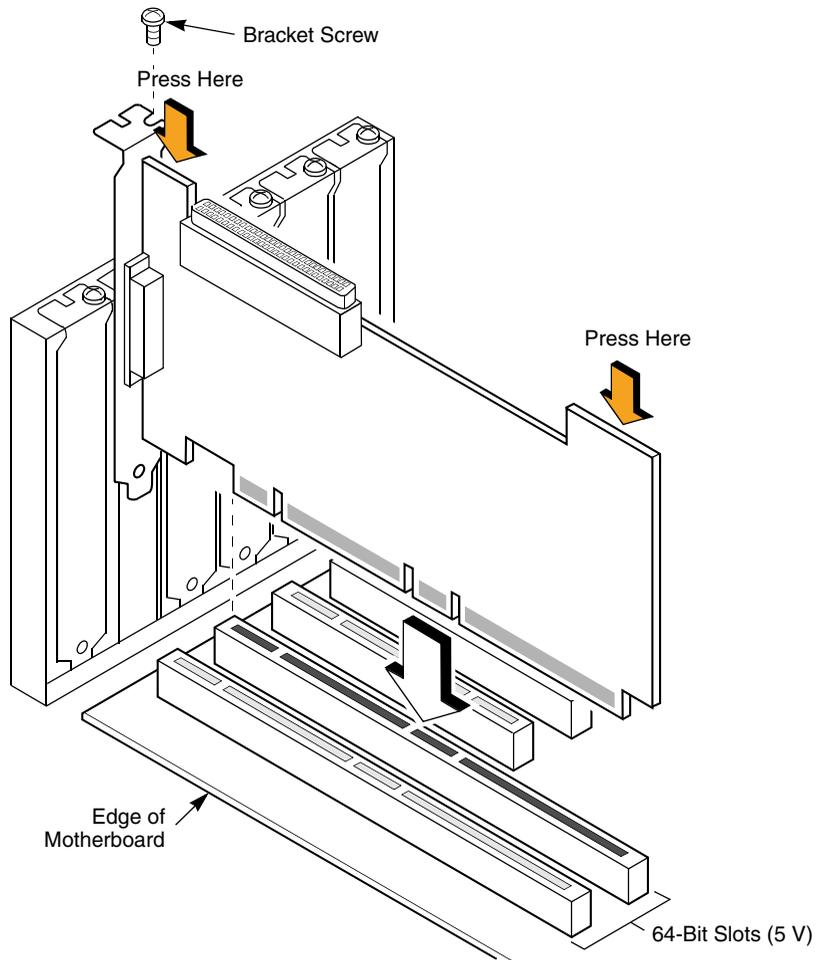
**Figure 2.2 Inserting the MegaRAID 320-2E Card in a PCI-Express Slot**
