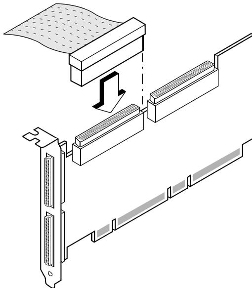
Step 2. Plug the 68-pin connector on the other end of the internal SCSI ribbon cable into the SCSI connector on the internal SCSI device, as shown in [Figure 2.10](#).
