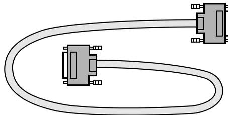
**Figure 2.7 SCSI Cable – 68-Pin VHDCI to 68-Pin HD**
