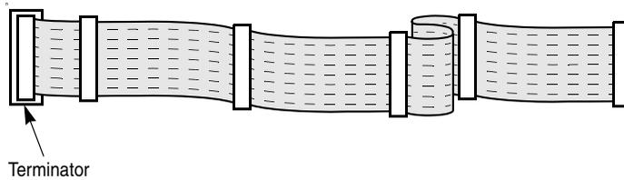
**Figure 2.5 SCSI Cable – 68-Pin High Density without Terminator**
