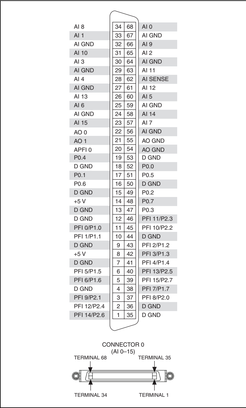
Figure A-59. USB-6281 Mass Termination Pinout
