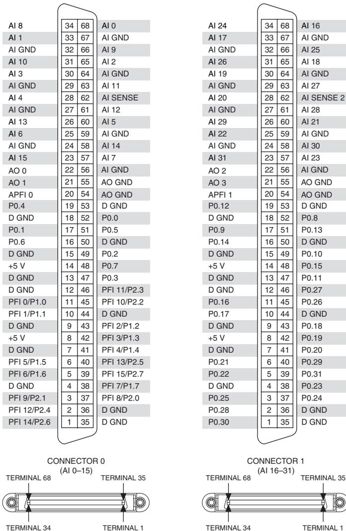
Figure 9. NI USB-6259 Mass Termination Pinout
