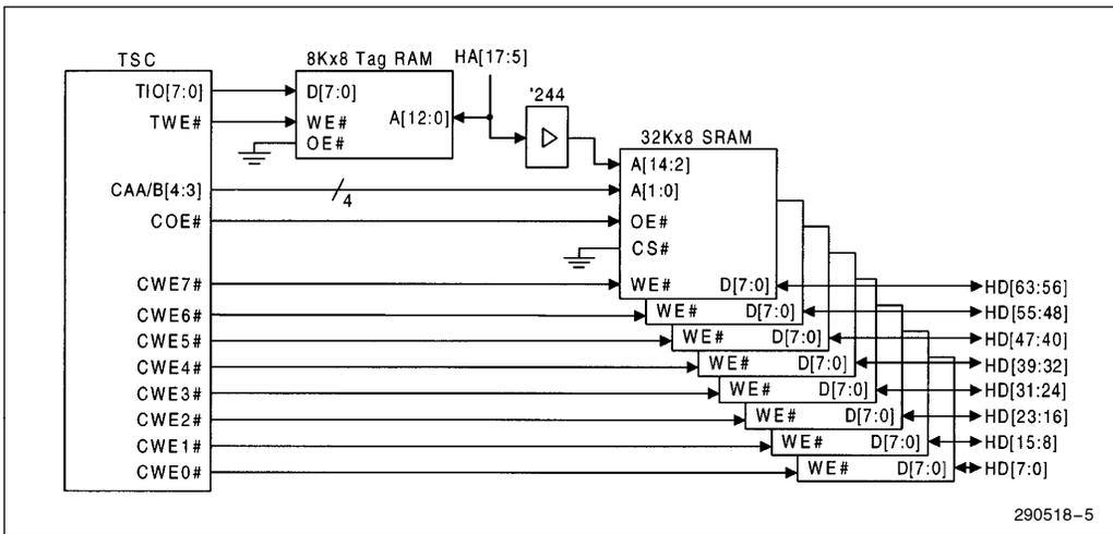
Figure 3. 256-Kbyte Second Level Cache (Standard SRAM)
