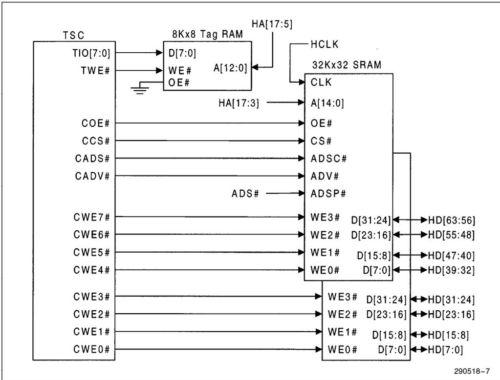
Figure 5. 256-Kbyte Second Level Cache (Burst SRAM)
