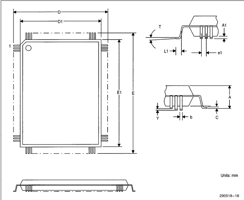
Figure 16. 100 Pin Plastic Quad Flat Pack (PQFP) Dimensions
