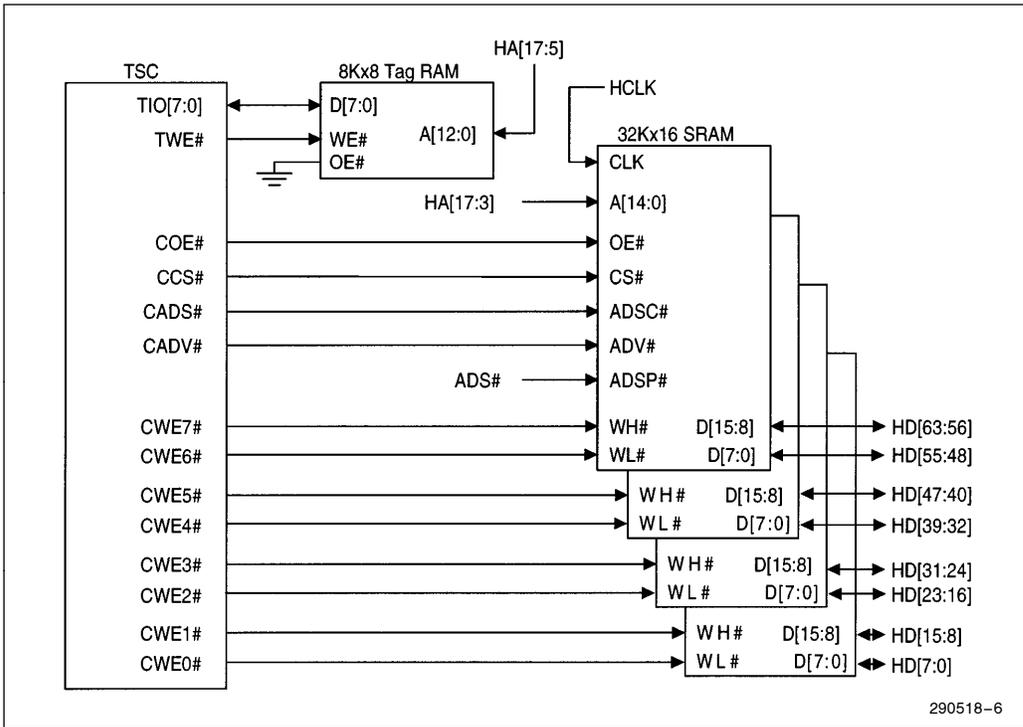
Figure 4. 256-Kbyte Second Level Cache (Burst SRAM)
