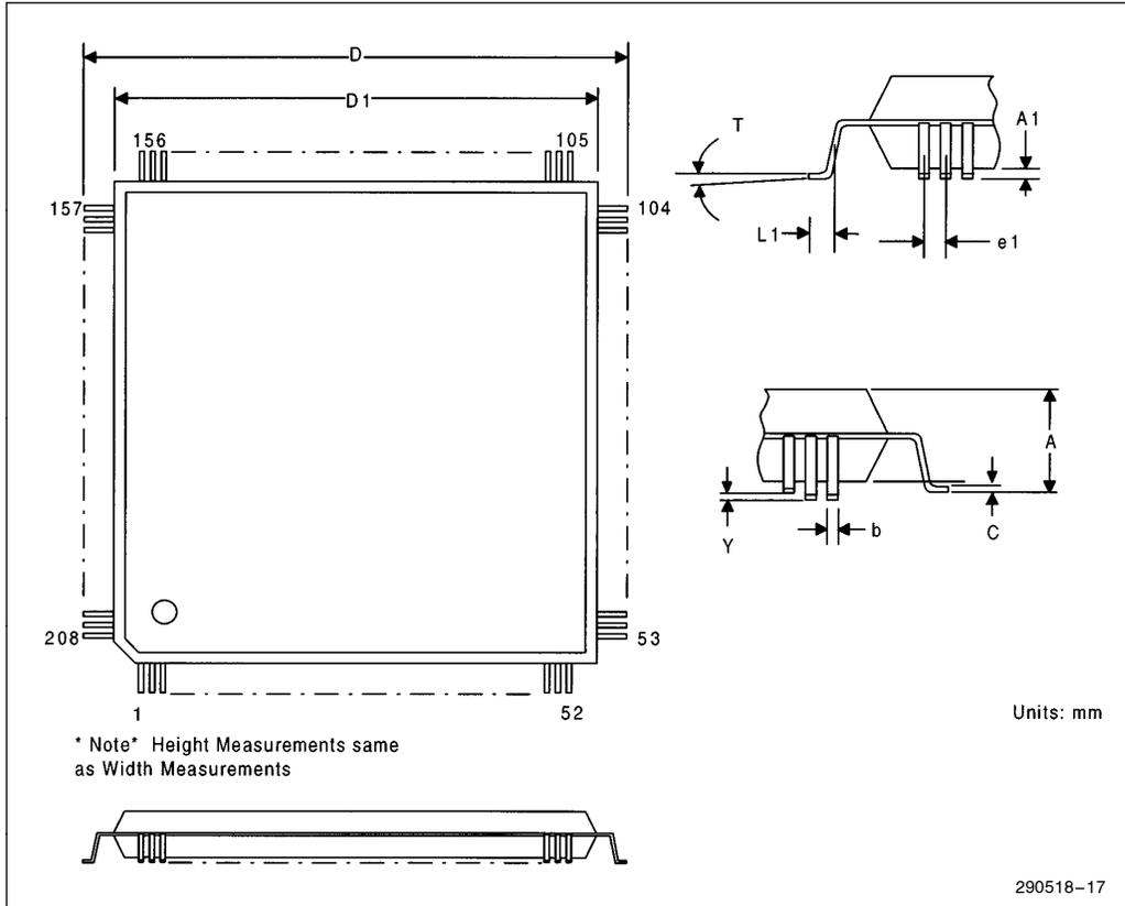
Figure 15. 208 Pin Quad Flat Pack (QFP) Dimensions
