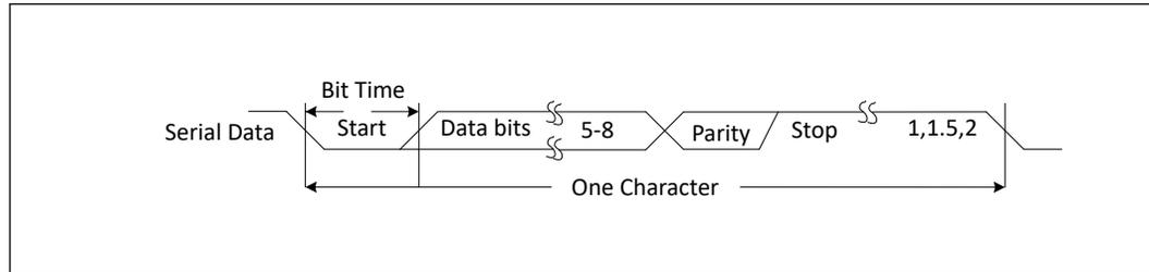
The UART Host Controller Line Control Register (LCR) is used to control the serial character characteristics. The individual bits of the data word are sent after the Start bit, starting with the least significant bit (LSB). These are followed by the optional parity bit, followed by the Stop bit(s), which can be 1, 1.5, or 2.
