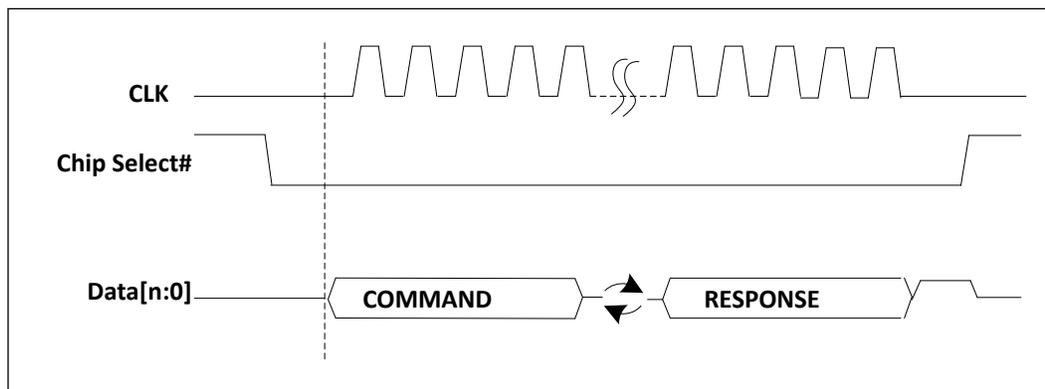
An eSPI transaction consists of a Command phase driven by the master, a turn-around phase (TAR), and a Response phase driven by the slave.
