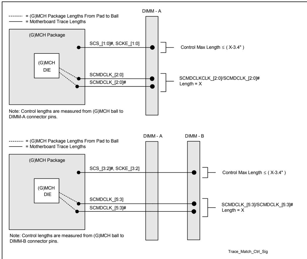
Figure 5-11. Control Group Bottom Layer to First DIMM Routing Example
