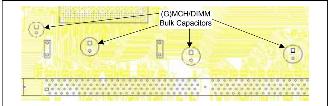
**Table 5-17. Intel® (G)MCH System Memory Bulk Capacitor Requirements**
