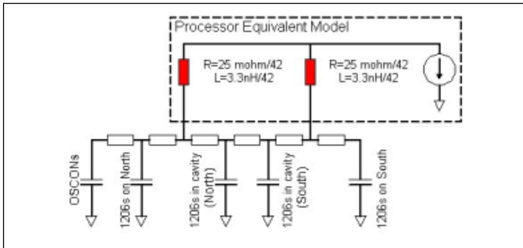
Table 4-20 lists model parameters for the system board shown in Figure 3-3. The values listed may be different depending on board layout.
