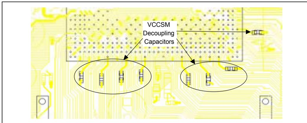
Figure 5-42. Intel® (G)MCH DDR 2.5 V Decoupling Capacitor Routing Alignment
