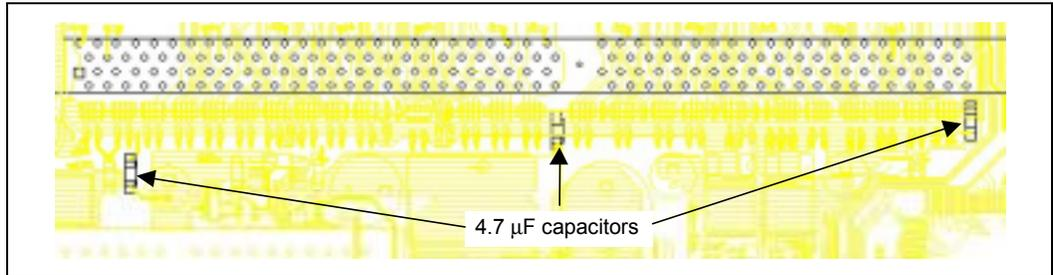
**Table 5-22. DDR VTT Termination Island High-Frequency Decoupling Requirements**
