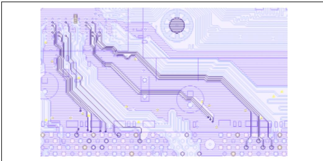
Figure 5-18. Address/Command Group Bottom Layer Routing Example
