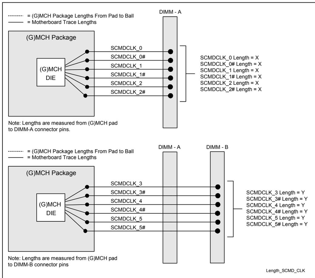
**Figure 5-35. Clock Pair Trace Length Matching Requirements**
