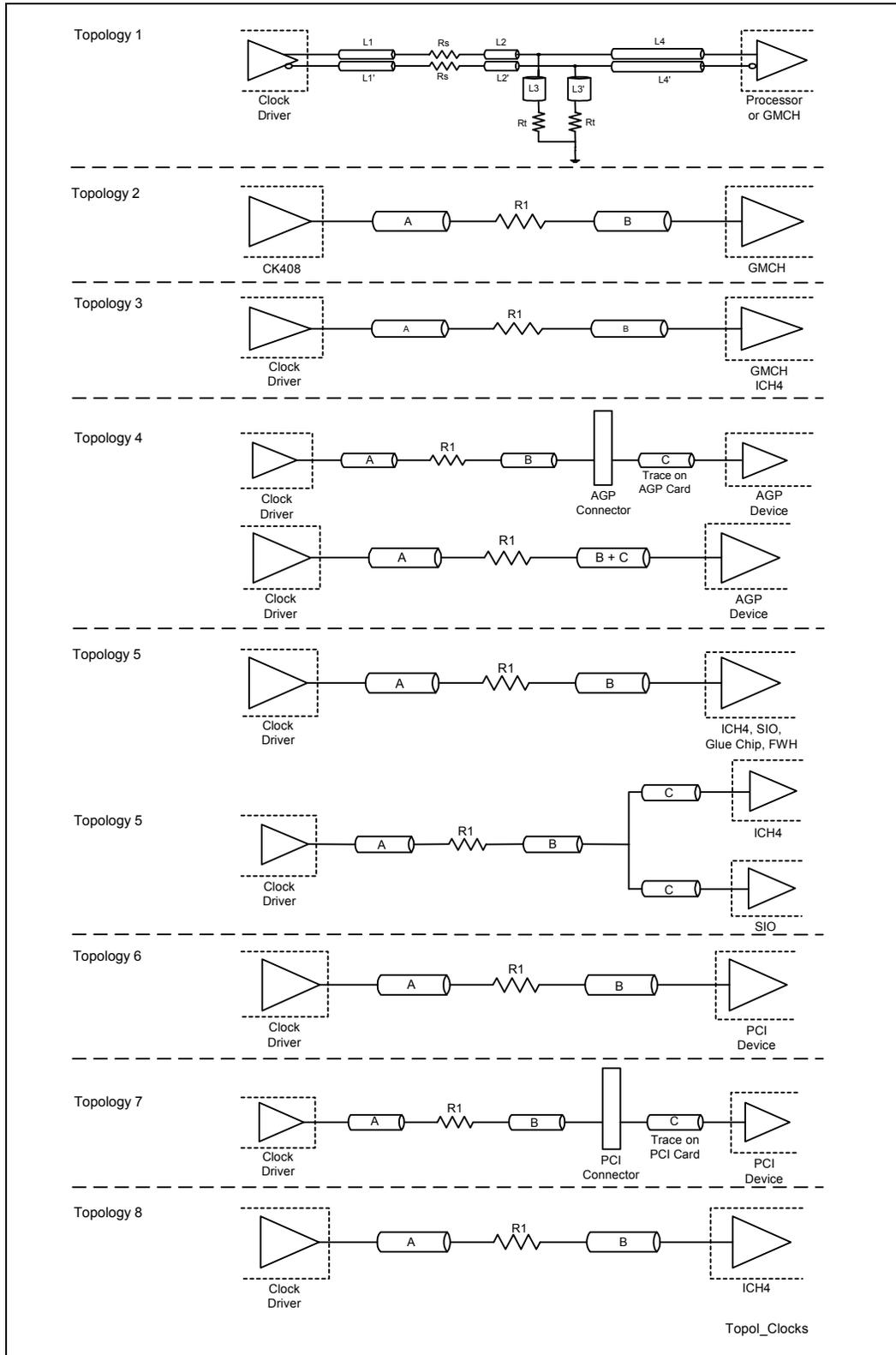
**Figure 16-5. Host Clocking Signals Routing Topologies**
