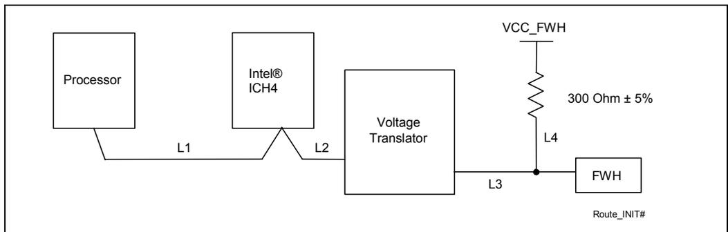
Level shifting is required for the INIT# signal to the FWH to meet the input logic levels of the FWH. Figure 4-8 illustrates one method of implementing this.
