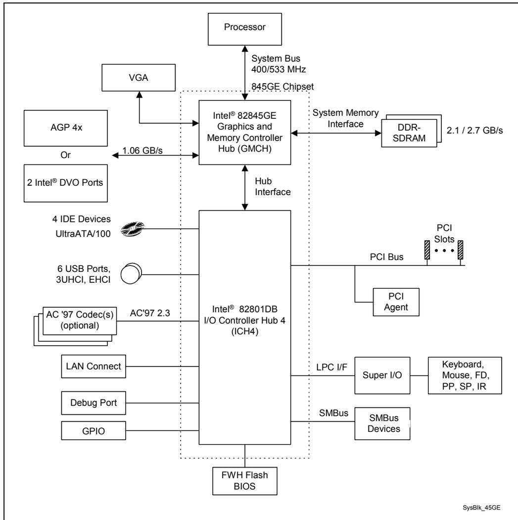
Figure 1-2 illustrates a typical Pentium 4 processor in the 478-pin package and 845PE chipset-based system configuration for mainstream desktop segments.
