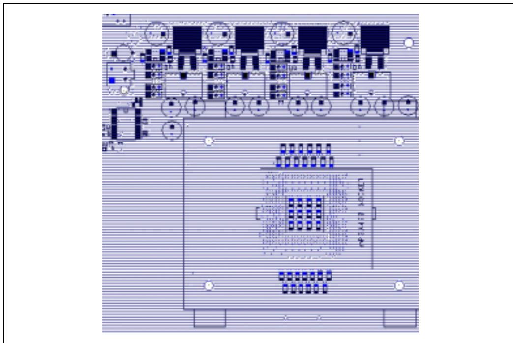
Figure 4-22. Bottom Layer Power Delivery Shape (VCC\_CPU)
