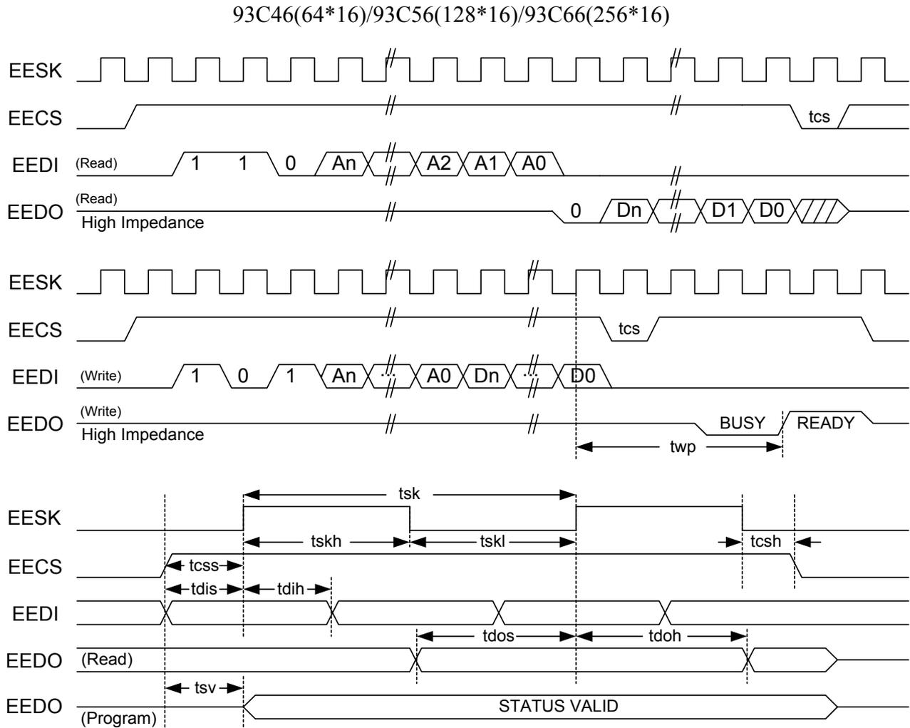
**Figure 12. Serial EEPROM Interface Timing**
