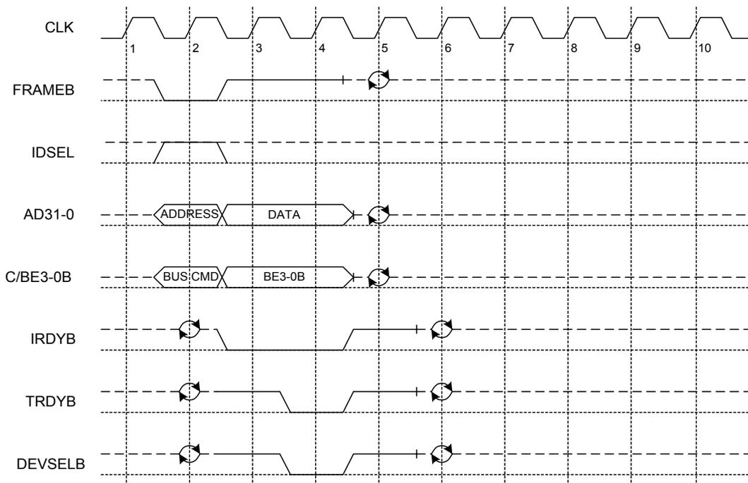
**Figure 20. Configuration Write**
