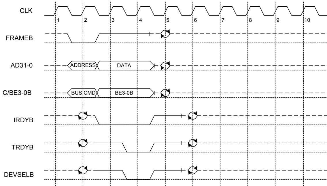
**Figure 18. I/O Write**
