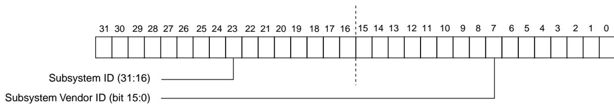
This register is used to uniquely identify the add-on board or subsystem where the NIC controller resides. Values in this register are loaded directly from external serial EEPROM after system reset automatically. Word location 36h of EEPROM is subsystem vendor ID and location 35h is sub-system ID.
