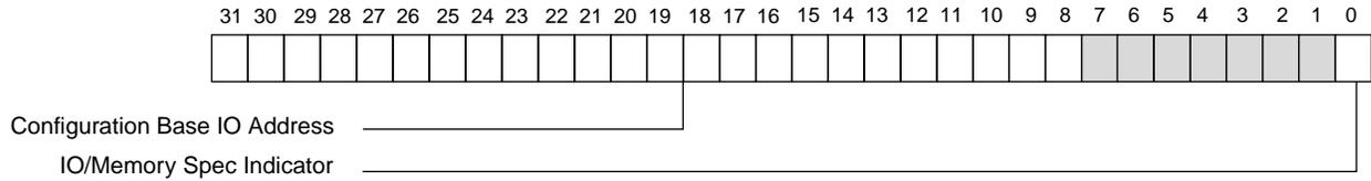
bit 0 : IO/Memory Space Indicator, fixed to 1 in this field will map into the IO space. This is a read only field.
