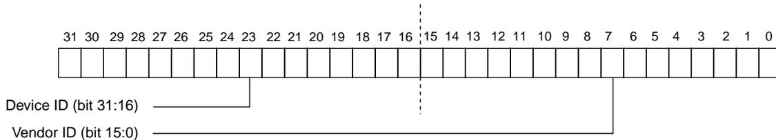
This register can be loaded from external serial EEPROM or use a MXIC preset value of "10D9" and "0531" for vendor ID and device ID respectively. Word location 3Eh and 3Dh in serial EEPROM are used to configure customer's vendor ID and device ID respectively. If location 3Eh contains "FFFF" value then MXIC's vendor ID and device ID will be set in this register, otherwise both 3Eh and 3Dh will be loaded into this register from serial EEPROM.
