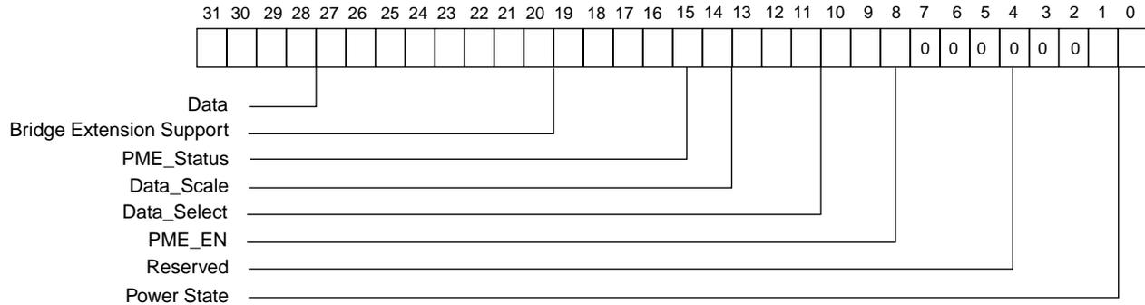
bit 1-0 : Power\_State, read/write, D0 mode is 00, D1 mode is 01, D2 mode is 10, D3 hot mode is 11.
