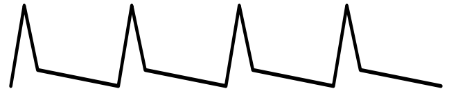
FIGURE 7. VOLTAGE ACROSS R WITHOUT RC
