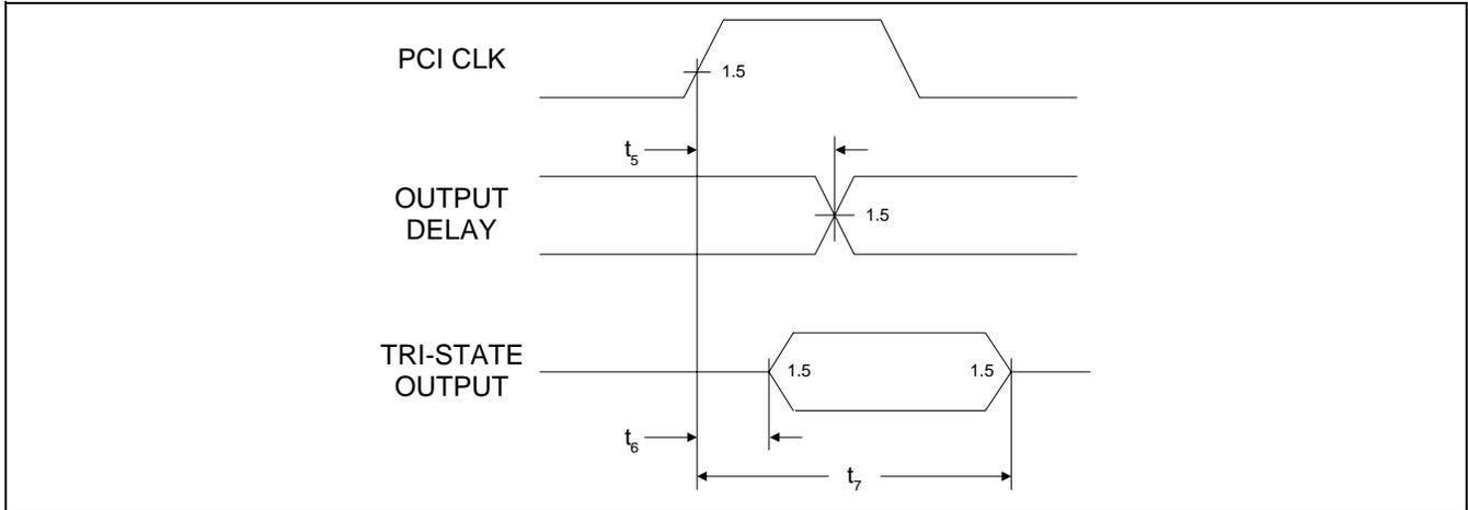
Figure 85. PCI Signal Input Timing
