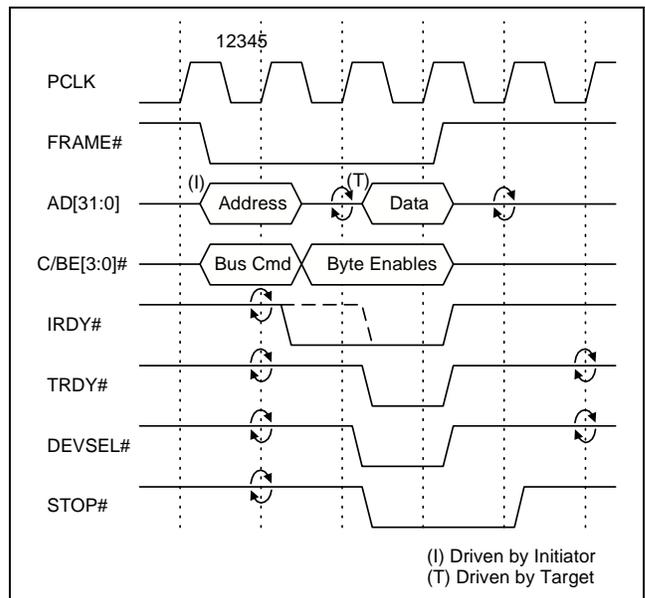
Figure 47. Burst PCI Bus Write of S5920 Registers
