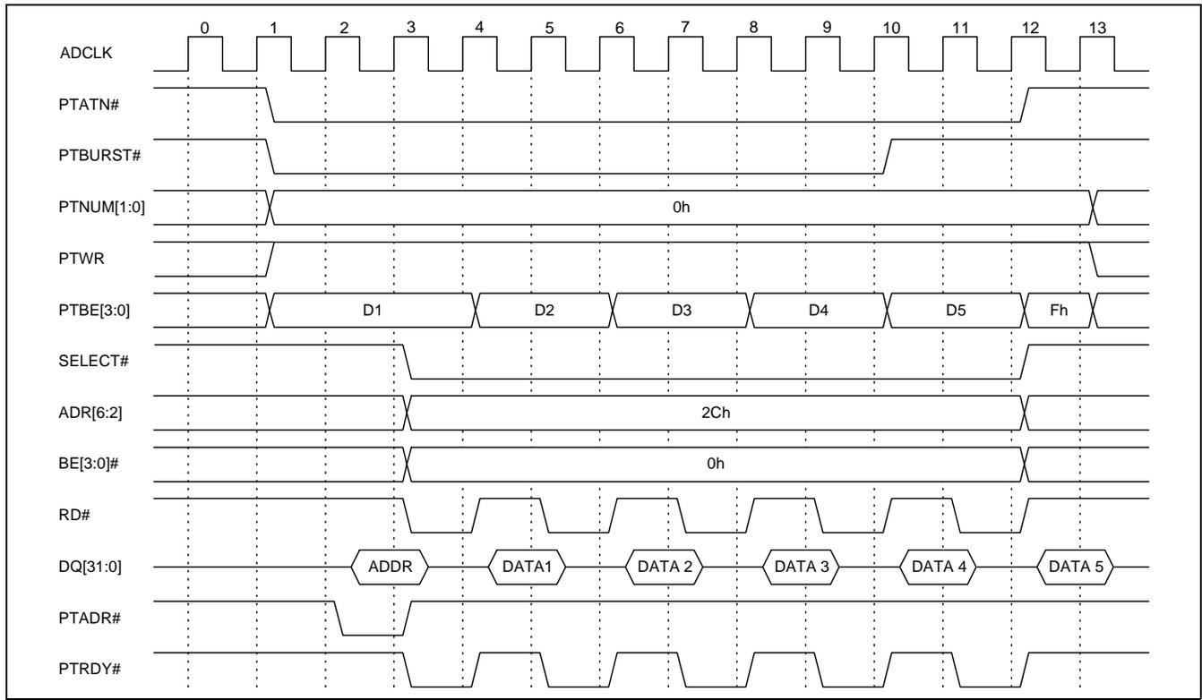
Figure 67. PCI to Add-On Passive Burst Read Access
