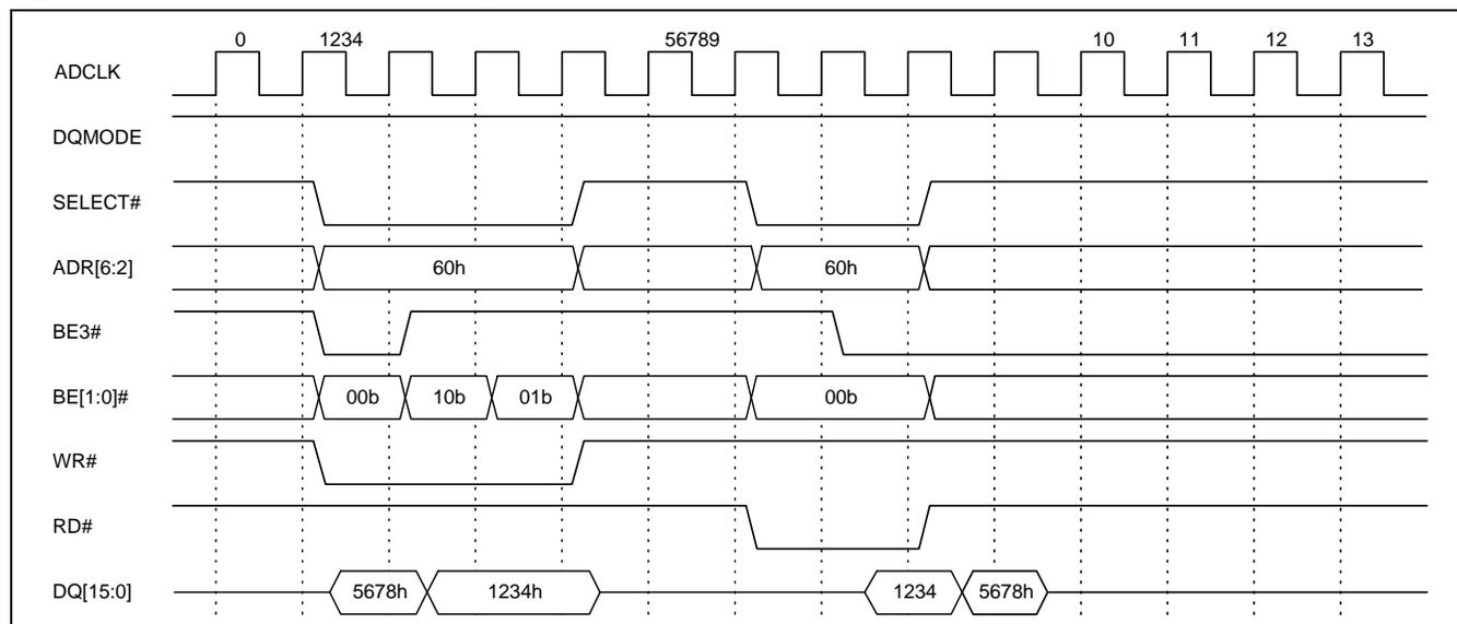
Figure 3. 16 Bit Mode Operation Register DWORD Write/Read Figure 3 shows an example of a DWORD write of 12345678h using a 16 bit-mode write transfer, and is described as follows:
