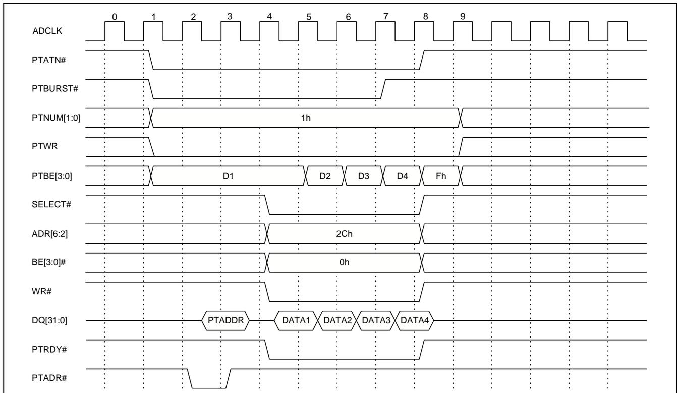
**Clock 1:** Pass-Thru signals PTATN#, PTBURST#, PTNUM[1:0], PTWR and PTBE[3:0] are driven to indicate what action is required by Add-On logic. These status signals are valid only when PTATN# is active. Add-On logic can decode status signals upon the assertion of PTATN#.
