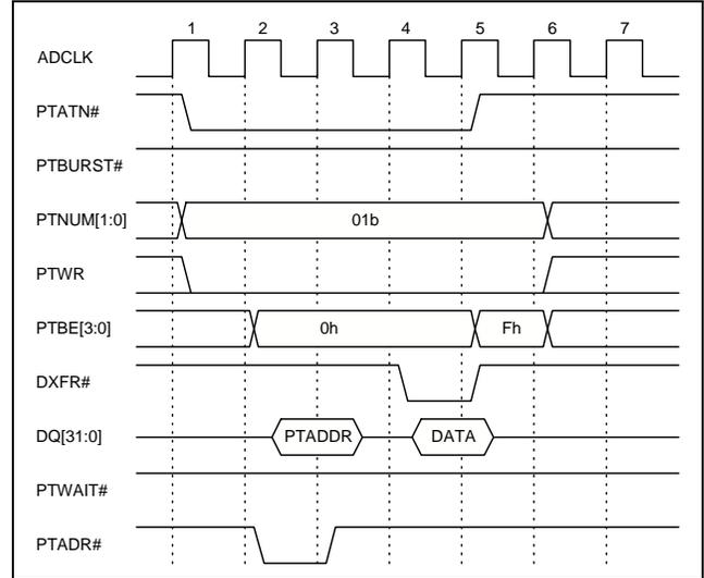
Figure 72. Active Mode PCI Read without PTADR#
