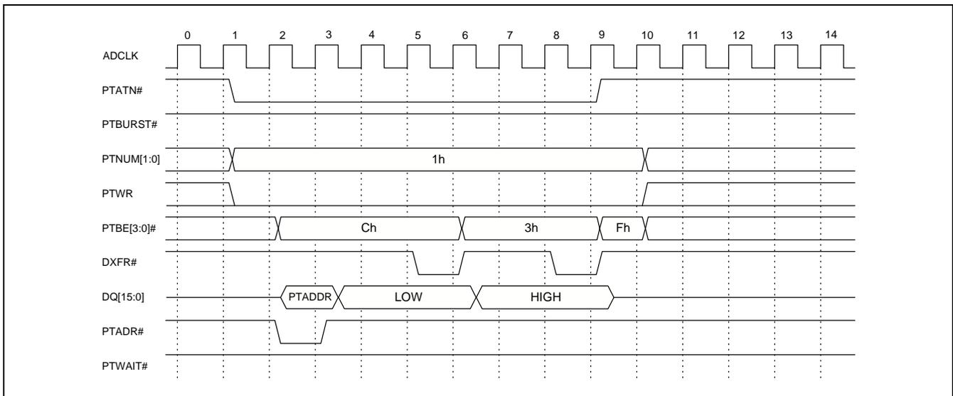
**Clock 2:** Since this region does not have PTADR# enabled as an output, it is driven active (low) and the PCI address for the current transaction is presented on the DQ[31:0] bus.
