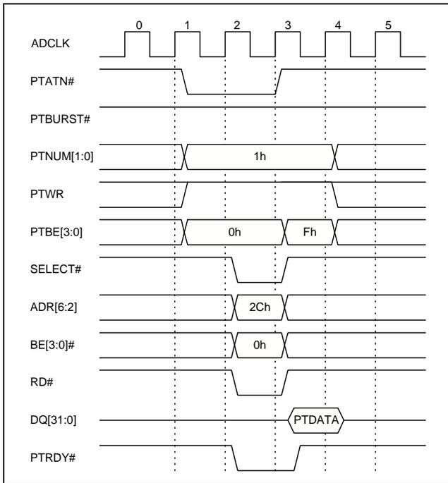
Figure 63. PCI To Add-On Passive Write w/Pass-Thru Address
