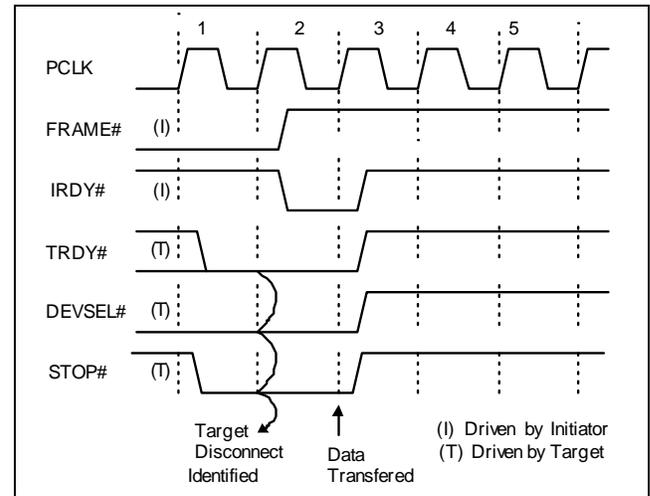
Figure 49. Figure 4b. Target Disconnect Example 2
