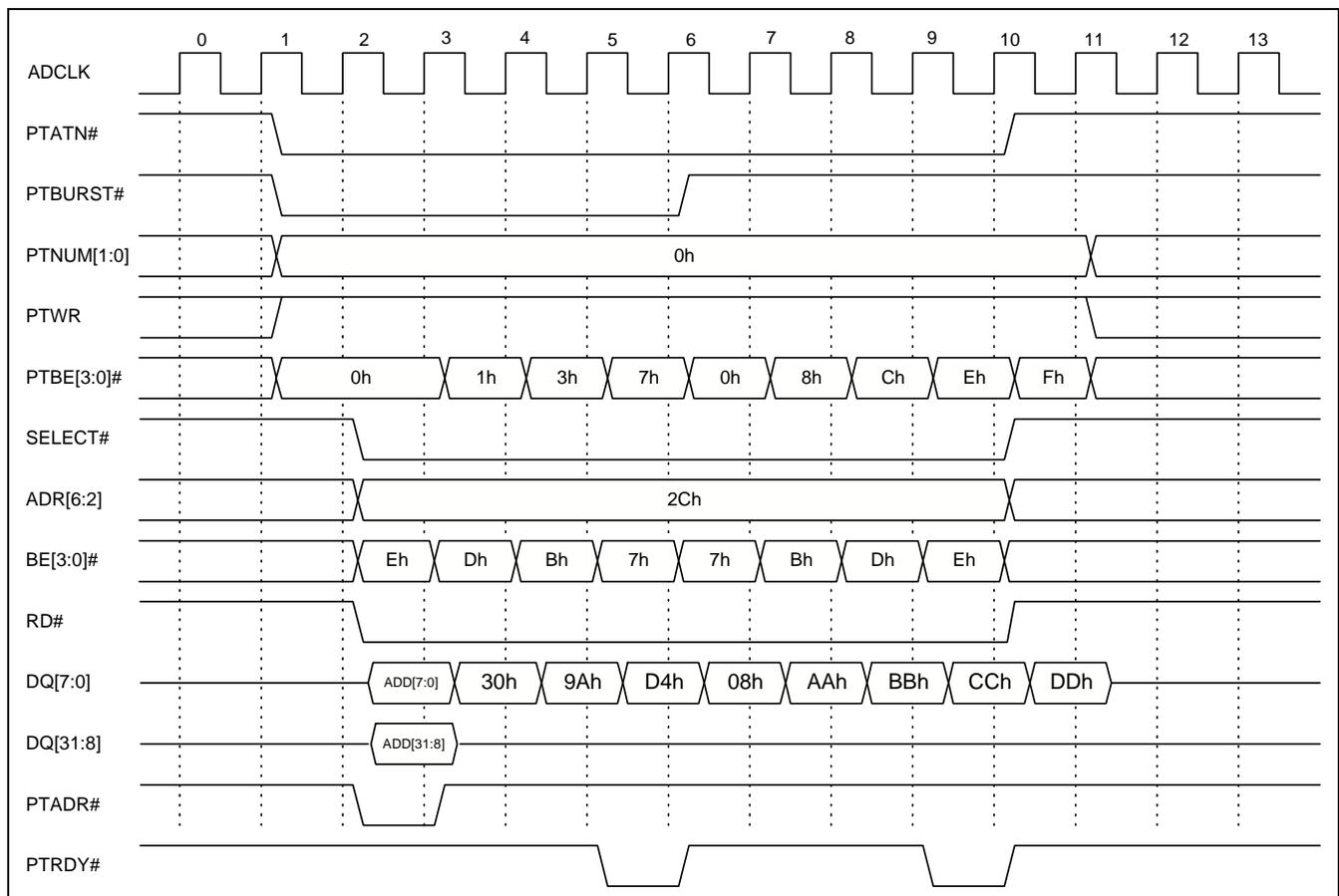
**Clock 5:** The Add-On logic latches BYTE1. RD# and BE2# are sampled asserted by the S5920, so BYTE2 of the APTD is driven on DQ[7:0] and PTBE2# is deasserted. The Add-On device asserts RD# and BE3#, thus requesting that BYTE3 of the APTD be driven on the DQ bus during the next cycle. PTRDY# is also asserted, indicating that the transfer is complete.
