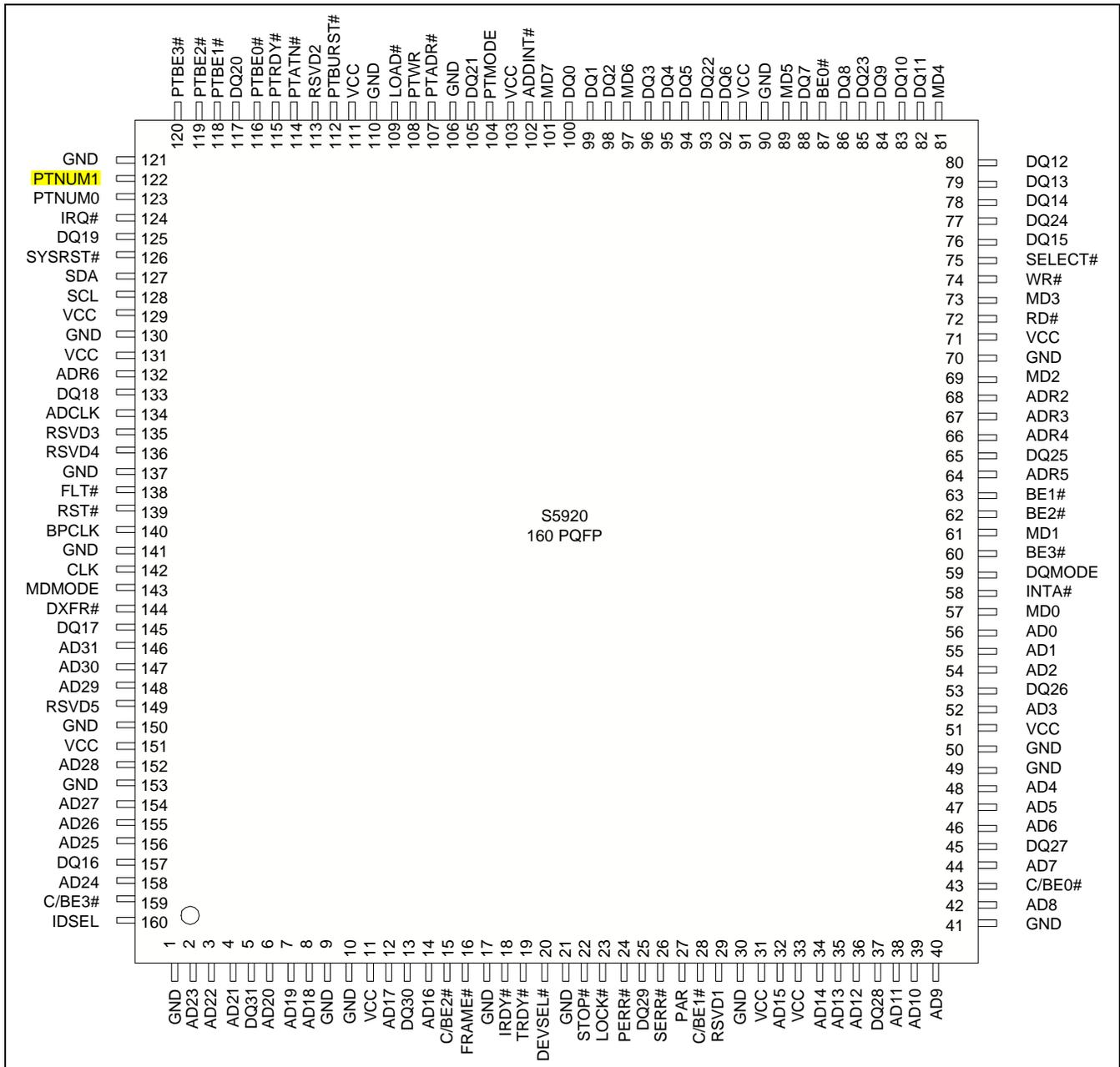
Figure 94. 160 PQFP (28 x 28 x 3.37 mm) - Plastic Quad Flat Package
