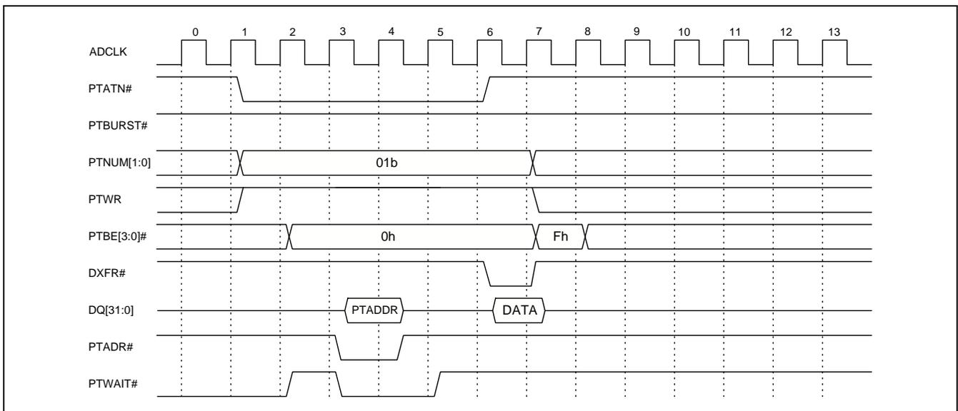
Figure 75. Active Mode 32-Bit PCI Write
