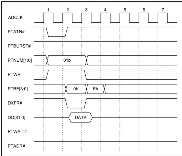
When PTADR# is active (low), the S5920 will drive the DQ[31:0] bus with the 32-bit PCI address regardless of the PTMODE pin. To avoid contention on the DQ[31:0] bus during PCI read cycles, the S5920 incorporates a turnaround cycle before starting to drive the data (DXFR# assertion). This is needed only when PTADR# is enabled and when zero wait states are programmed during a Pass-Thru read cycle. The cycle immediately following the address cycle will be a turnaround cycle as shown in Figure 13a.
