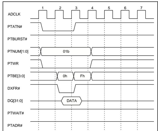
The PTADR# signal is controlled by the most significant bit of every region control field in the PTCR register. If this bit is zero then the PTADR# pin is not driven at the start of an Active mode transfer. If this bit is set to one, the PTADR# pin will be enabled and driven active (low) for one and only one clock after PTATN# was sampled active provided PTWAIT# was also sampled high.
