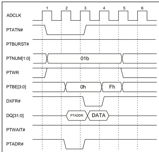
The address phase of a Pass-Thru consists of the cycles from PTATN# asserted through PTADR# asserted (if PTADR# has been programmed to be disabled, there is no address phase). If PTWAIT# is asserted before the address phase, the address phase is delayed. The address phase will occur during the cycle after the clock edge that PTWAIT# is sampled high and PTATN# is sampled low.
