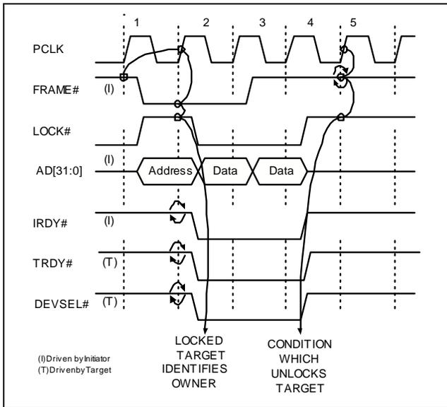
Figure 53. Access Attempt to a Locked Target
