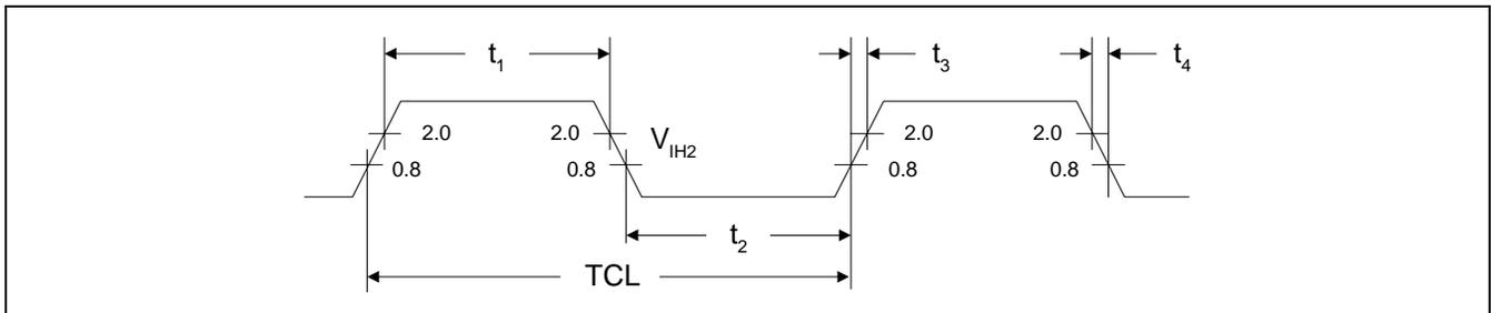
Figures 2 and 3 define the conditions under which timing measurements are made. The user designs must guarantee that minimum timings are met with maximum clock skew rate (fastest edge) and voltage swing.
