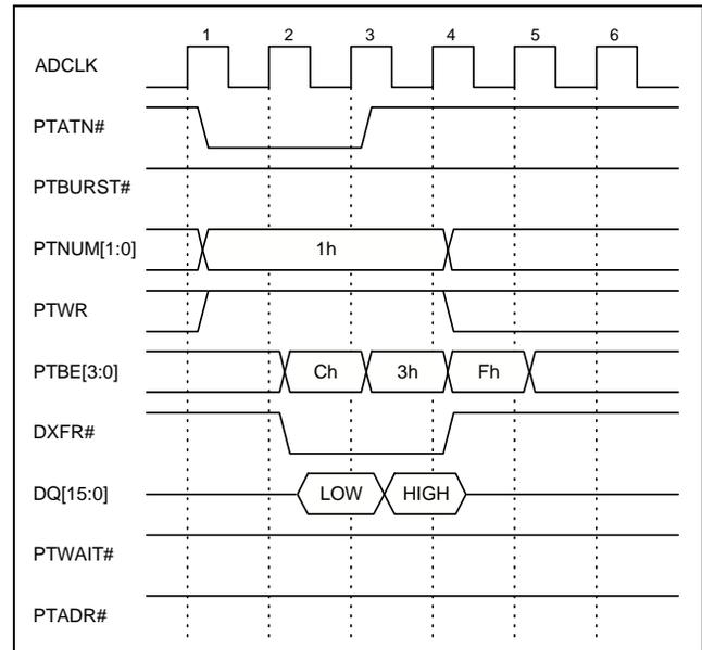
Figure 22 shows a Pass-Thru write cycle with 0 wait states for an 8-bit region. The PTBE[3:0]# signals are used by the Add-On device to determine validity of the current byte cycle and also, which byte of a long word is currently being driven by the S5920. PTADR# is enabled as an output.
