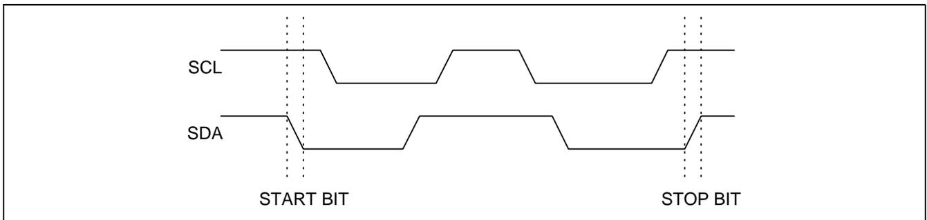
Figure 38. Serial Interface Clock Data Relationship
