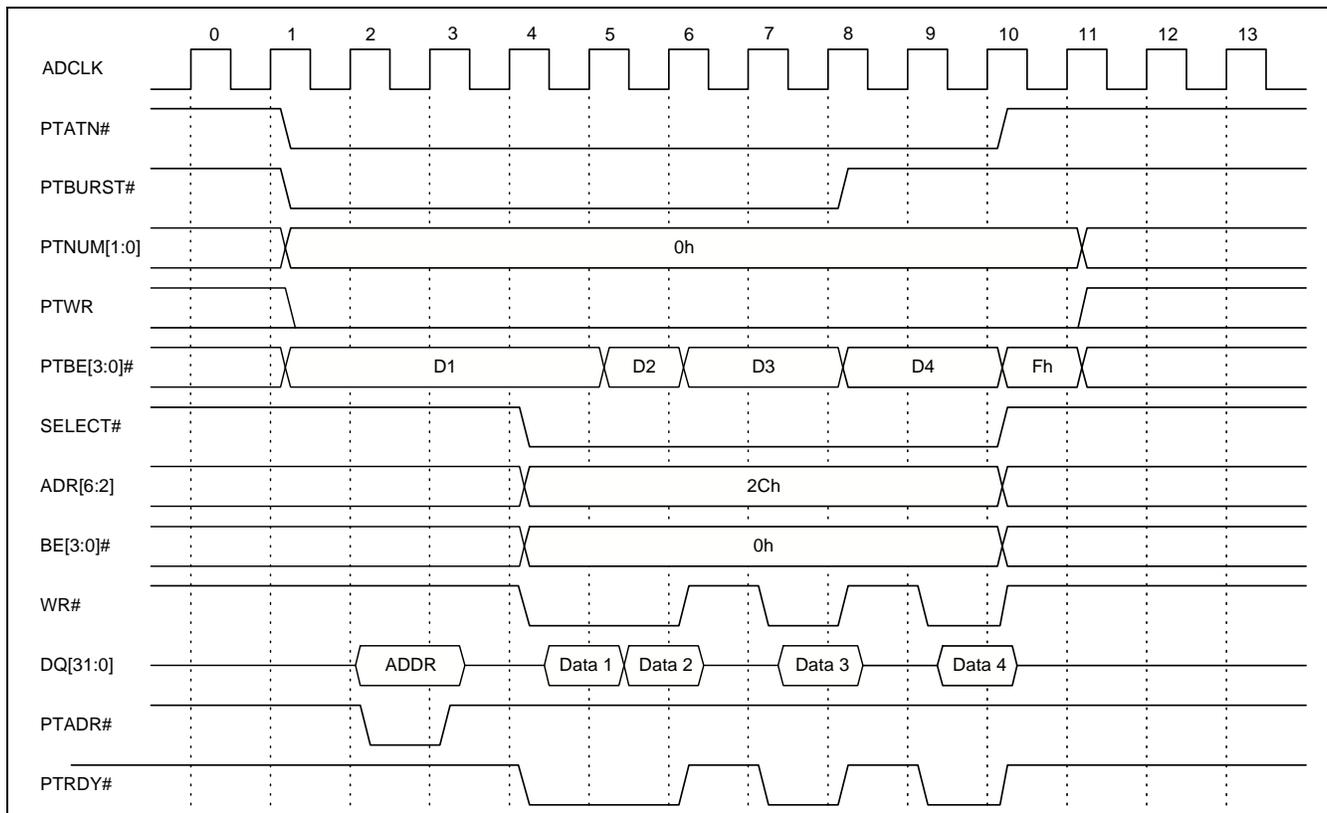
Figure 9 shows a Passive Mode Pass-Thru burst read access (Add-On write) of four DWORDs, using PTADR# to provide an address-phase.
