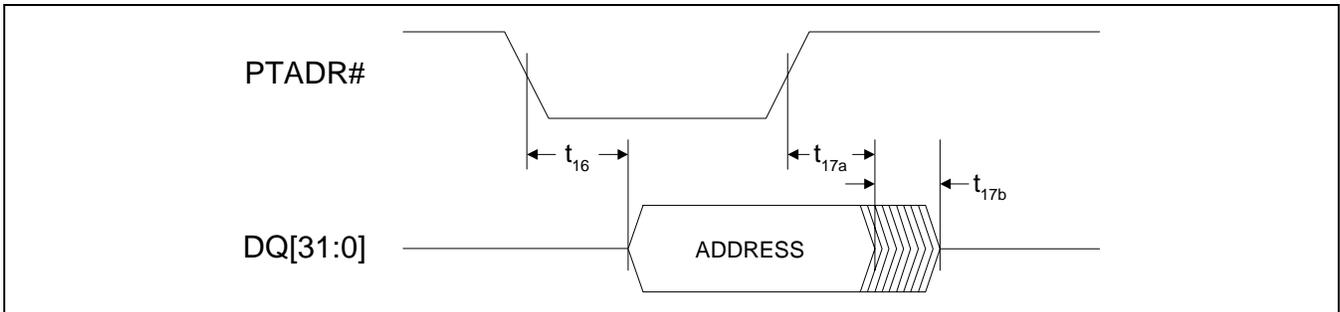
Figure 89. Passive Mode Pass-Thru Operation
