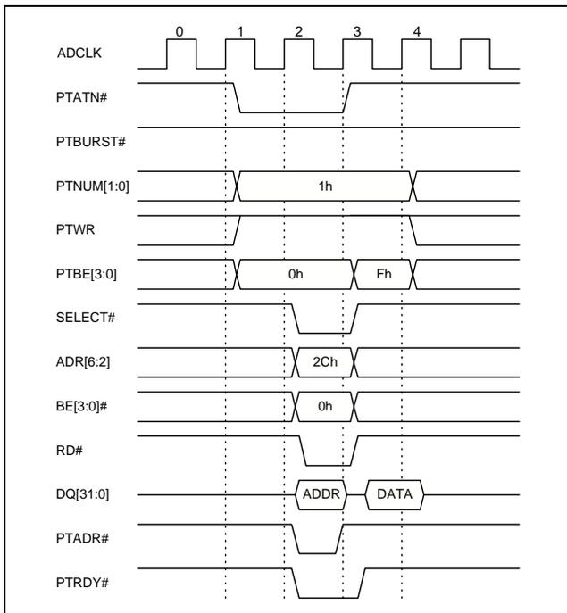
Clock 0: The address is recognized as a PCI write to Pass-Thru region 1. The PCI bus write address is stored in the Pass-Thru Address Register. The PCI bus write data is stored in the S5920 Write FIFO. Add-On bus signals PTATN#, PTBURST#, PTNUM[1:0],
