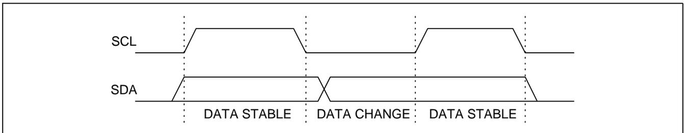
Figure 39. Serial Interface Byte Access-Write
