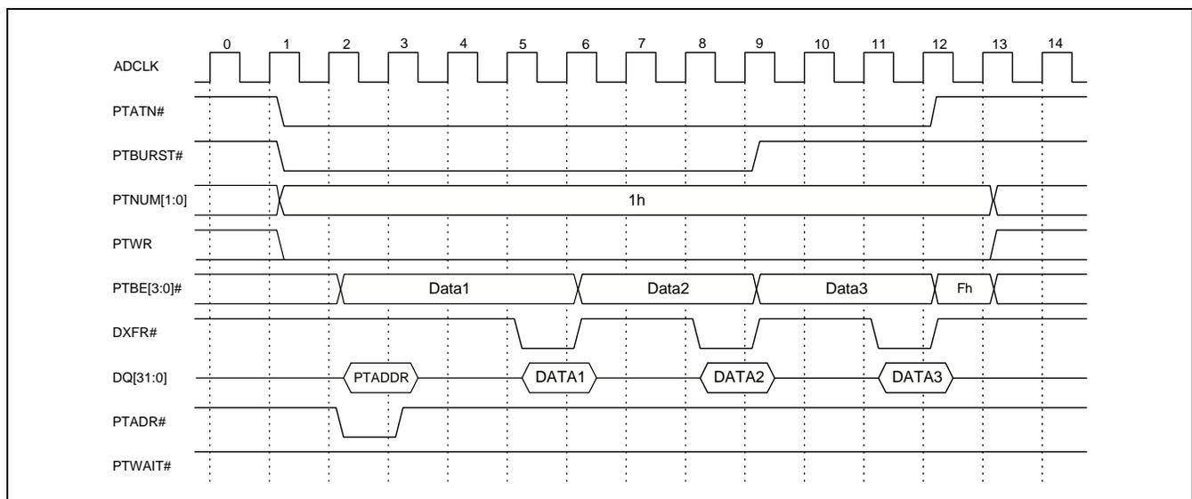
Figure 80. Active Mode PCI Read
