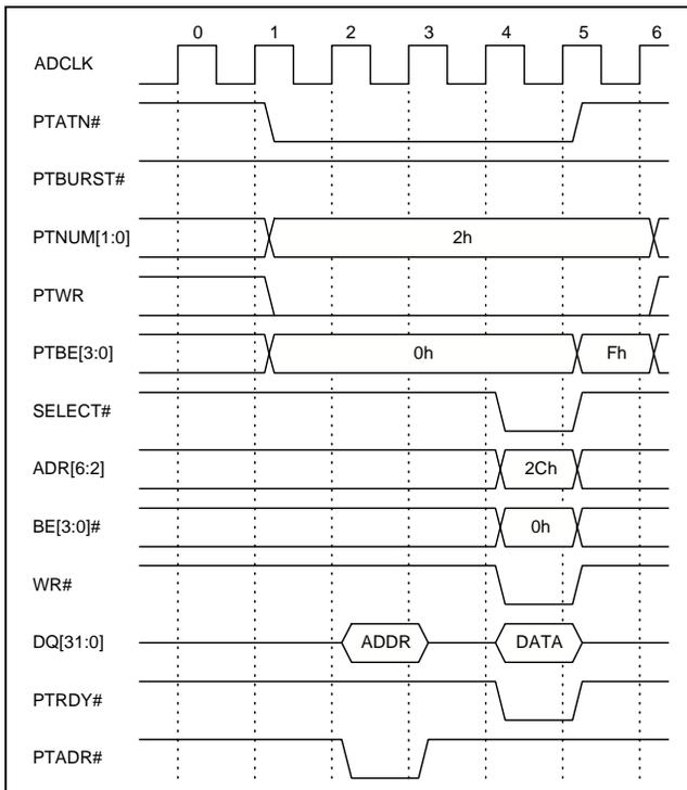
**Clock 0:** The address is recognized as a PCI read of Pass-Thru region 2. The PCI bus read address is stored in the Pass-Thru Address Register. Add-On bus signals PTATN#, PTBURST#, PTNUM[1:0], PTWR and PTBE[3:0] will update on the next rising edge of ADCLK.
