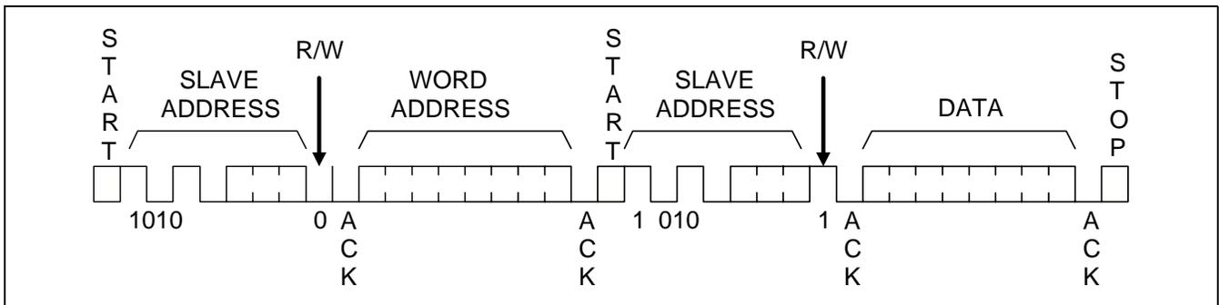
Figure 41. Serial Byte Access- Sequential Read
