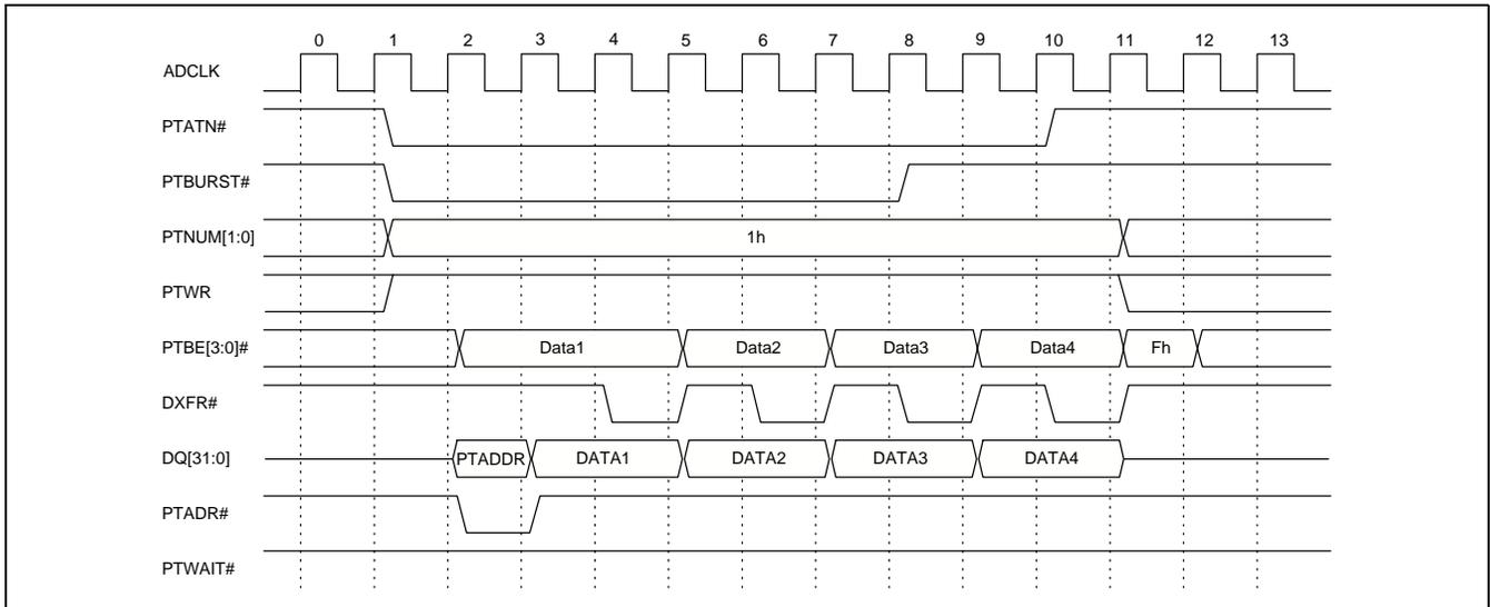
Figure 78. 16-Bit Active Mode PCI Read w/ Programmed Wait States
