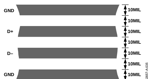
Figure 35. Arrangement of Signal Tracks
