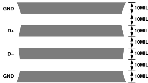
Figure 18. Arrangement of Signal Tracks
